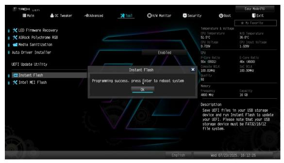
11. After the system restarts, press [F2] to enter the BIOS setup utility during boot up. In Exit menu, please select "Load UEFI Defaults "and press [Enter] to continue. Select "Save Changes and Exit "and press [Enter] to exit the BIOS setup utility. Now, the system is booting up with new BIOS.
