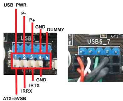
Step3. Install Multi-Angle CIR Receiver to the front USB port. If Multi-Angle CIR Receiver cannot successfully receive the infrared signals from MCE Remote Controller, please try to install it to the other front USB port.
