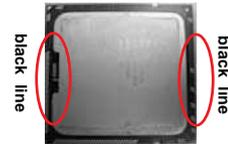
Step 3-2. Orient the CPU with IHS (Integrated Heat Sink) up. Locate Pin1 and the two orientation key notches.
