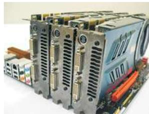
Step2. Connect the auxiliary power source to the PCI Express graphics card. Please make sure that both power connectors on the PCI Express graphics card are connected. Repeat this step on the three graphics cards.
