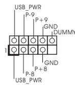
Besides seven default USB 2.0 ports on the I/O panel, there are three USB 2.0 headers on this motherboard. USB8\_9 and USB6\_7 headers can support four USB 2.0 ports (two ports for each header). USB10 header can support one USB 2.0 port.
