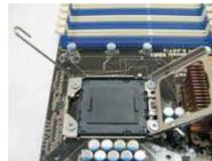
Step 2. Remove PnP Cap (Pick and Place Cap).
