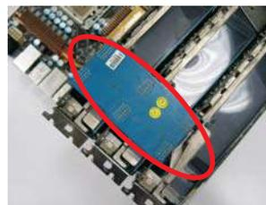
Step4. Connect a VGA cable or a DVI cable to the monitor connector or the DVI connector of the graphics card that is inserted to PCIE1 slot.
