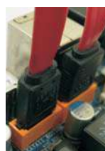
Connect the SATA data cables to both orange eSATAII connectors (eSATAII_BOTTOM and eSATAII_TOP)
