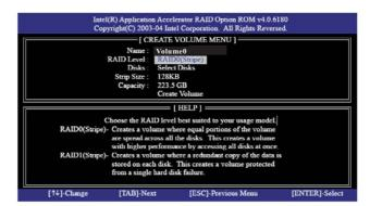
Use the up or down arrow keys to select your desired **RAID Level**. You may select RAID0 (Stripe), RAID1 (Mirror), RAID 5, RAID 10, or Matrix Storage for your RAID level. Press <Enter>, and then you can select **Strip Size**.
