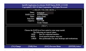
If you selected RAID 0 (Stripe), use the up or down arrow keys to select the stripe size for your RAID 0 array then press <Enter>.The available values range from 8 KB to 128 KB. The default selection is 128 KB. The strip value should be chosen based on the planned drive usage.
