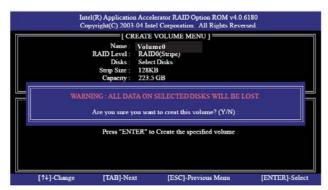
Press <Y> to complete the setup of RAID.
