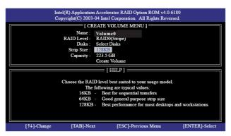
If you selected RAID 0 (Stripe), use the up or down arrow keys to select the stripe size for your RAID 0 array then press <Enter>.The available values range from 8 KB to 128 KB. The default selection is 128 KB. The strip value should be chosen based on the planned drive usage.
