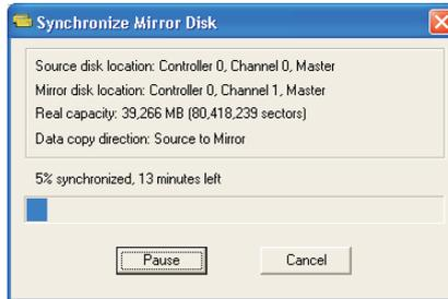
When the synchronization starts, a dialog will show the process. You can pause or cancel this process at any time. If you cancel the synchronization process, the RAID is on "need-sync" condition. You should synchronize again to guarantee the data are identical between the source and the mirror disk drives.
