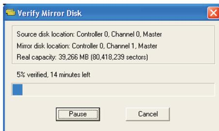
3. When the mirror disk is not identical with the corresponding source disk, the mirror disk will be marked with a “need-sync” icon:
