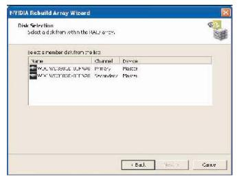
E. Select the drive that you want to rebuild by clicking it from the list, then click Next. The Completing the NVIDIA Rebuild Array page appears.
