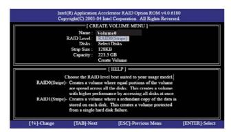
Use the up or down arrow keys to select your desired **RAID Level**. You may select RAID0 (Stripe), RAID1 (Mirror), RAID 5, RAID 10, or Rapid Storage for your RAID level. Press <Enter>, and then you can select **Strip Size**.
