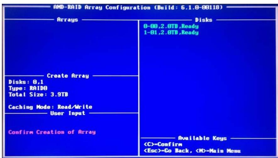
When completed, you will see the new array on the main screen. Press <Esc> to exit the RAID BIOS utility.
