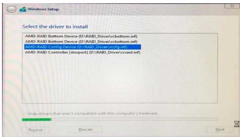
I. After RAID driver is loaded, the RAID disk will show up.
