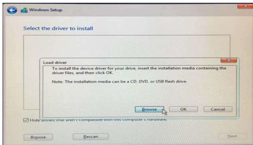
C. For 32bit OS, the driver is under /I386 directory. For 64bit OS, the driver is under /AMD64 directly. Please select the correct driver for your Windows version (Windows 10).
