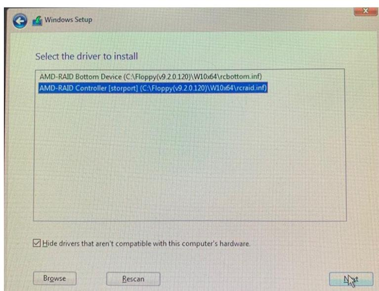
F. After RAID driver is loaded, the RAID disk will show up. Load the Third driver.
