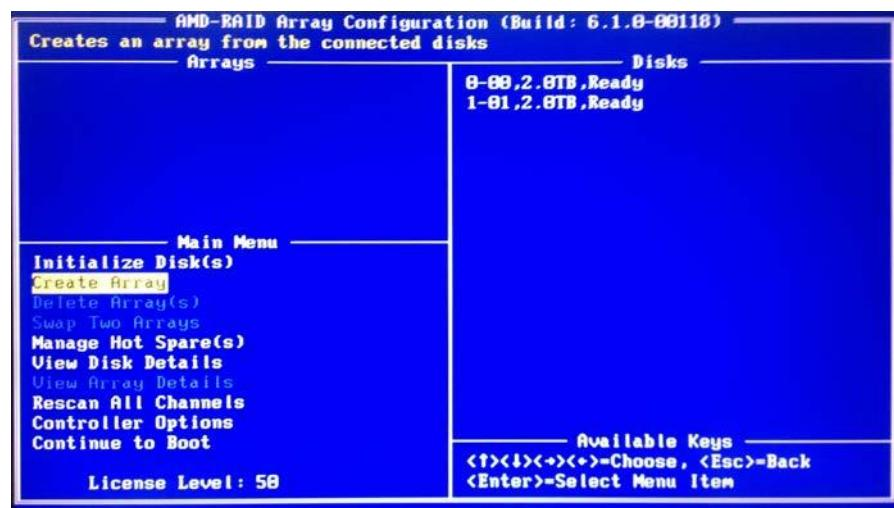
Use the arrow keys to select the hard drives to be included in the RAID array and press <Ins>. The selected hard drives will be shown in green. To use all of the hard drives, simply press <A> to select all. Then press <Enter>.
