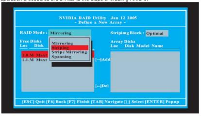
Striping block size is given in kilobytes, and affect how data is arranged on the disk. It is recommended to leave this value at the default Optimal, which is 64KB, but the values can be between 8KB and 128KB (8, 16, 32, 64, and 128KB). Then, you have to assign the disks. The disks that you enabled from the RAID Config BIOS setup page appear in the Free Disks block. These are the drives that are available for use as RAID array disk,
