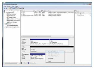
Right-click on the unallocated partition and select New Simple Volume. Follow the Wizard for setting up and formatting the partition. Once that is done, you can start using the newly created stripped array.
