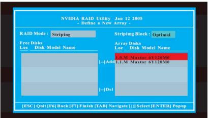
After assigning your RAID array disks, press <F7> to save your changes of RAID array disks.
