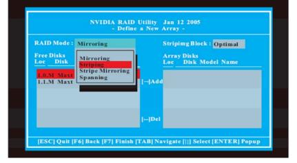
Striping block size is given in kilobytes, and affect how data is arranged on the disk. It is recommended to leave this value at the default Optimal, which is 64KB, but the values can be between 8KB and 128KB (8, 16, 32, 64, and 128KB). Then, you have to assign the disks. The disks that you enabled from the RAID Config BIOS setup page appear in the Free Disks block. These are the drives that are available for use as RAID array disk,
