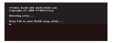
After rebooting your computer, wait until you see the RAID software prompting you to press <F10>. The RAID prompt appears as a part of the system POST and boot process prior to loading the OS. You have a few seconds to press <F10> before the window disappears.
