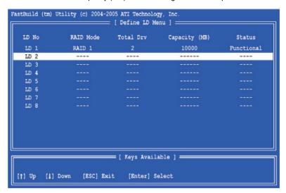
2. Press the up and down arrow keys to select an available logical drive number and press <Enter>.
