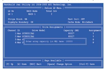
1. Enter the desired capacity (MB) for the first logical drive and press <Enter>. The Define LD Menu displays again.
