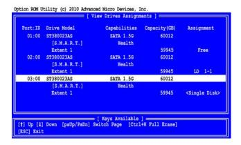
2 Press the arrow keys to highlight a physical drive you want to secure erase and press Ctrl-H. The caution screen appears.
