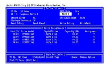
Choose the RAID Level you want. In the Define LD Menu section, press the Spacebar to toggle through logical drive types:
