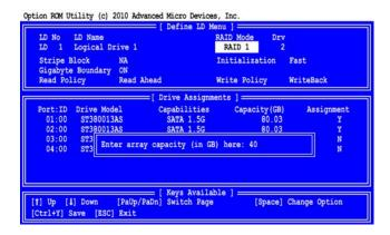
2 Enter the desired capacity in GB for the first logical drive and press Enter. The Define LD Menu displays again.
