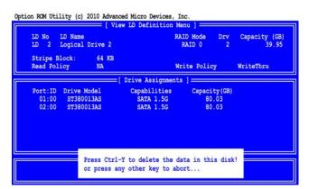
3 Press Ctrl-Y to confirm and complete logical drive deletion.
