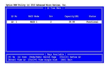
3 Press the up and down arrow keys to select an available logical drive number and press Enter.
