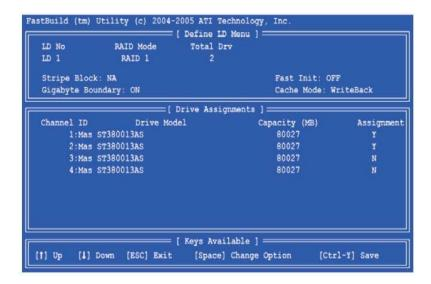
Choose the RAID level you want. In the Define LD Menu section, press the spacebar to cycle through logical drive types, including RAID 0, RAID 1, RAID Ready, JBOD and RAID 10.
