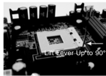
STEP 1: Lift The Socket Lever Up to 90°
