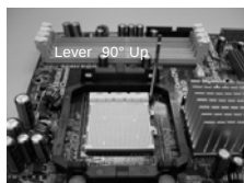
STEP 1: Lift Up The Socket Lever
