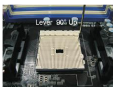
STEP 1: Lift Up The Socket Lever
