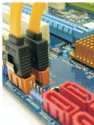
Connect the SATA data cables to both orange SATAII connectors (SATAII_6 (Port 5) and SATAII_5 (Port 4))
