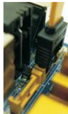
Connect the SATA data cable to one of the orange eSATAII connector (eSATAII_BOTTOM (Port 5))
