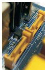
eSATAII connectors (eSATAII_TOP (Port 4) and eSATAII_BOTTOM (Port 5))
