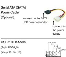
Please connect the black end of SATA power cable to the power connector on each drive. Then connect the white end of SATA power cable to the power connector of the power supply.
