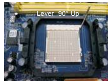
STEP 1: Lift Up The Socket Lever
