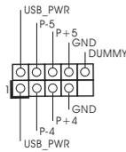
ASRock 8CH I/O accommodates 4 default USB 2.0 ports. If those USB 2.0 ports on the I/O panel are not sufficient, this USB 2.0 header is available to support 2 additional USB 2.0 ports.
