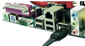
Connect the other end of the eSATAII device cable to eSATAII port of the I/O shield
