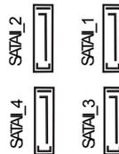
These Serial ATAII (SATAII) connectors support SATAII or SATA hard disk for internal storage devices. The current SATAII interface allows up to 3.0 Gb/s data transfer rate.
