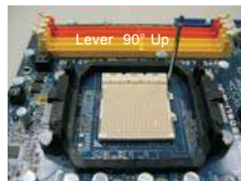
STEP 1: Lift Up The Socket Lever
