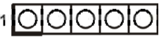
20 : COM Port Pin9 PWR Setting Jumpers PWR_COM1 ~ 6 (For COM Port1 ~ 6) 1-2: +5V 2-3: +12V
