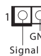
23 : Chassis Intrusion Headers C11: Close: Active Case Open Open: Normal C12: Close: Normal Open: Active Case Open
