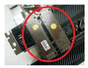
Step4. Connect a VGA cable or a DVI cable to the monitor connector or the DVI connector of the graphics card that is inserted to PCIE2 slot.
