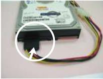
**Step 4** Connect SATA data cable to the SATA2 HDD.
