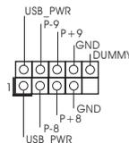
Besides four default USB 2.0 ports on the I/O panel, there are three USB 2.0 headers on this motherboard. Each USB 2.0 header can support two USB 2.0 ports.
