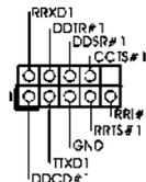
This COM1 header supports a serial port module.
