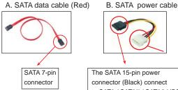
The SATA 15-pin power connector (Black) connect to SATA / SATAII / SATA3 HDD
