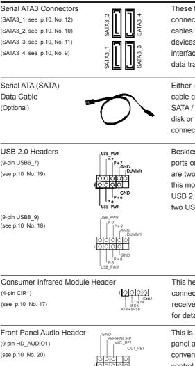
These four Serial ATA3 (SATA3) connectors support SATA data cables for internal storage devices. The current SATA3 interface allows up to 6.0 Gb/s data transfer rate.
