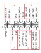
This header supports multiple functions on the front panel, including the front panel SMB, internet status indicator and chassis intrusion pin.
