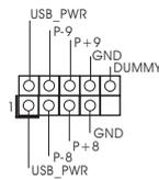
Besides six default USB 2.0 ports on the I/O panel, there are two USB 2.0 headers on this motherboard. Each USB 2.0 header can support two USB 2.0 ports.
