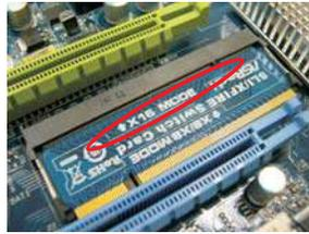
Step 3. To change it to CrossFire Mode, you need to reverse the direction of ASRock SLI/XFire Switch Card. Please simultaneously pull open both the retention arms that hold the card in position. The card itself will spring away from the retention slot. Take it out gently by holding its edges, and keep away from touching the connectors (Golden Fingers).
