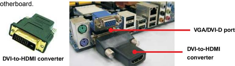
2. If you connect the DVI-to-HDMI converter to the VGA/DVI-D port, please connect the HDMI monitor cable to the DVI-to-HDMI converter. If you don't connect the DVI-to-HDMI converter to the VGA/DVI-D port, please connect the DVI-D monitor cable to the VGA/DVI-D port. And connect the D-Sub monitor cable to the VGA/D-Sub port.
