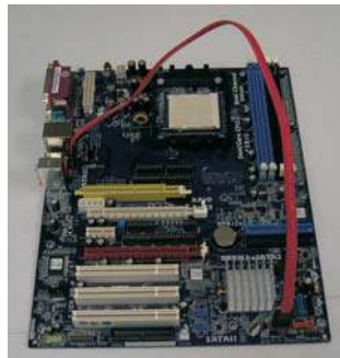
Connect the SATA data cable to the red eSATAII connector (eSATAII_BOTTOM)
