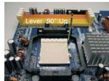
STEP 1: Lift Up The Socket Lever
