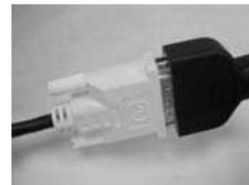
Connect the DVI-DMS cable to the monitor connector.
