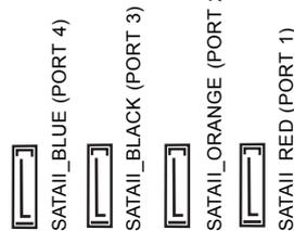
These four Serial ATAII (SATAII) connectors support SATA data cables for internal storage devices. The current SATAII interface allows up to 3.0 Gb/s data transfer rate.
