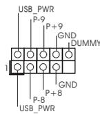
Besides two default USB 2.0 ports on the I/O panel, there are four USB 2.0 headers on this motherboard. Each USB 2.0 header can support two USB 2.0 ports.
