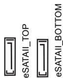
These two eSATAII connectors support SATA data cables for external SATAII function. The current eSATAII interface allows up to 3.0 Gb/s data transfer rate.
