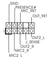
This is an interface for the front panel audio cable that allows convenient connection and control of audio devices.
