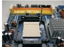
STEP 1: Lift Up The Socket Lever
