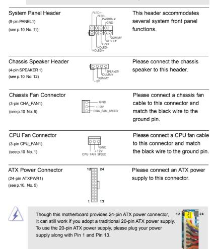
20-Pin ATX Power Supply Installation
