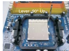
STEP 1: Lift Up The Socket Lever
