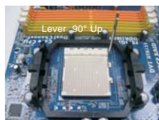
STEP 1: Lift Up The Socket Lever
