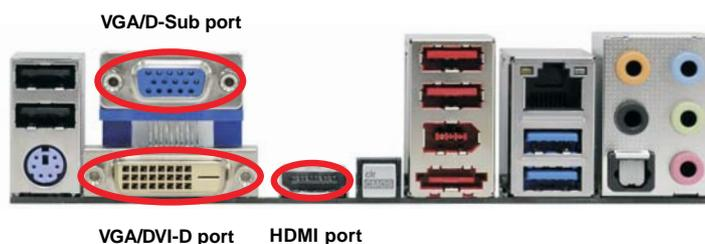
2. If you have installed onboard VGA driver from our support CD to your system already, you can freely enjoy the benefits of dual monitor function after your system boots. If you haven't installed onboard VGA driver yet, please install onboard VGA driver from our support CD to your system and restart your computer. Then you can start to use dual monitor function on this motherboard.
