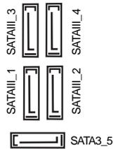
These five Serial ATA3 (SATA3) connectors support SATA data cables for internal storage devices. The current SATA3 interface allows up to 6.0 Gb/s data transfer rate.
