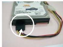
**Step 4** Connect SATA data cable to the SATA3 HDD.
