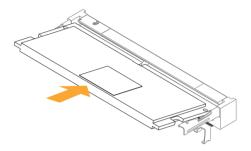
Step 2. Firmly insert the SO-DIMM into the slot until the retaining clip at both ends fully snaps back in place and the SO-DIMM is properly seated.
