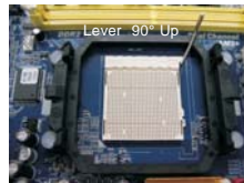
STEP 1: Lift Up The Socket Lever
